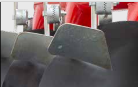
Mud Scraper Adjustable mud scrapers are placed in the machines so as to prevent accumulation of the mud.
